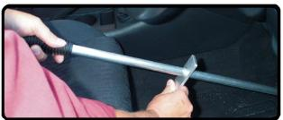
4. Angle the plate on the tube so that it locks in place, ensuring sufficient force is maintained on the Brake Pedal.
