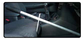
5. To release the device, hold the grip, apply downward pressure, "square up" the oblong plate and slide away from the seat pad.
