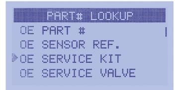
TPMS Go guides you to compatible sensors and part numbers for any vehicle, and indicates the correct torque values.
