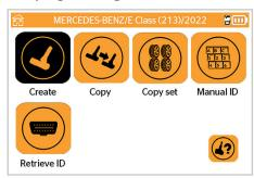
Programming of universal sensors can be done quickly, either wheel by wheel – or even for the entire set of tires at the same time, ideal for winter wheels. Subsequent relearning with the OBDII interface takes less than 90 seconds.
