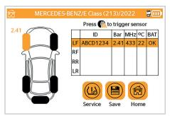
TPMS sensors can be checked quickly and easily on the vehicle. All the sensor information such as sensor ID, pressure, frequency and temperature status is also displayed and can be saved as a report.
