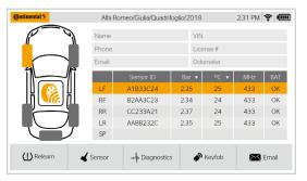
The vehicle screen is used for reading the sensor information – the customer information is acquired at the vehicle. All the sensor information such as sensor ID, pressure, frequency and temperature status is also displayed and can be saved as a report.
