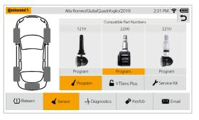
Programming of universal sensors can be done quickly, either wheel by wheel – or even for the entire set of tires at the same time, ideal for winter wheels. Subsequent relearning with the OBDII interface takes less than 90 seconds.
