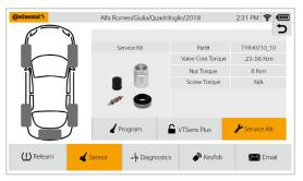
You can use the Service Kit function to view spare part numbers and torques for sensor valves. A picture of the kit is also displayed to prevent possible identification errors.
