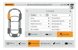
The Tire Inspection function allows you to check each tire and rim, enter notes about any damage or suggestions, measure tire tread depth and record DOT information. Tapping the camera icon also lets you take pictures for documentation purposes.
