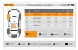
The vehicle screen is used for reading the sensor information - the customer information is acquired at the vehicle. All the sensor information such as sensor ID, pressure, frequency and temperature status is also displayed and can be saved as a report.
