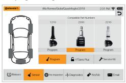
Programming of universal sensors can be done quickly, either wheel by wheel - or even for the entire set of tires at the same time, ideal for winter wheels. Subsequent relearning with the OBDII interface takes less than 90 seconds.
