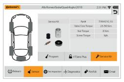
You can use the Service Kit function to view spare part numbers and torques for sensor valves. A picture of the kit is also displayed to prevent possible identification errors.
