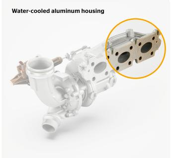
Water cooling enables the use of the lightweight material aluminum and makes the turbine housing almost 30% lighter and significantly more durable.
