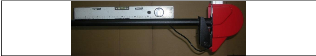
Figure F6.13: Square the external sensor using a level. Tighten the 3 M6 screws.
