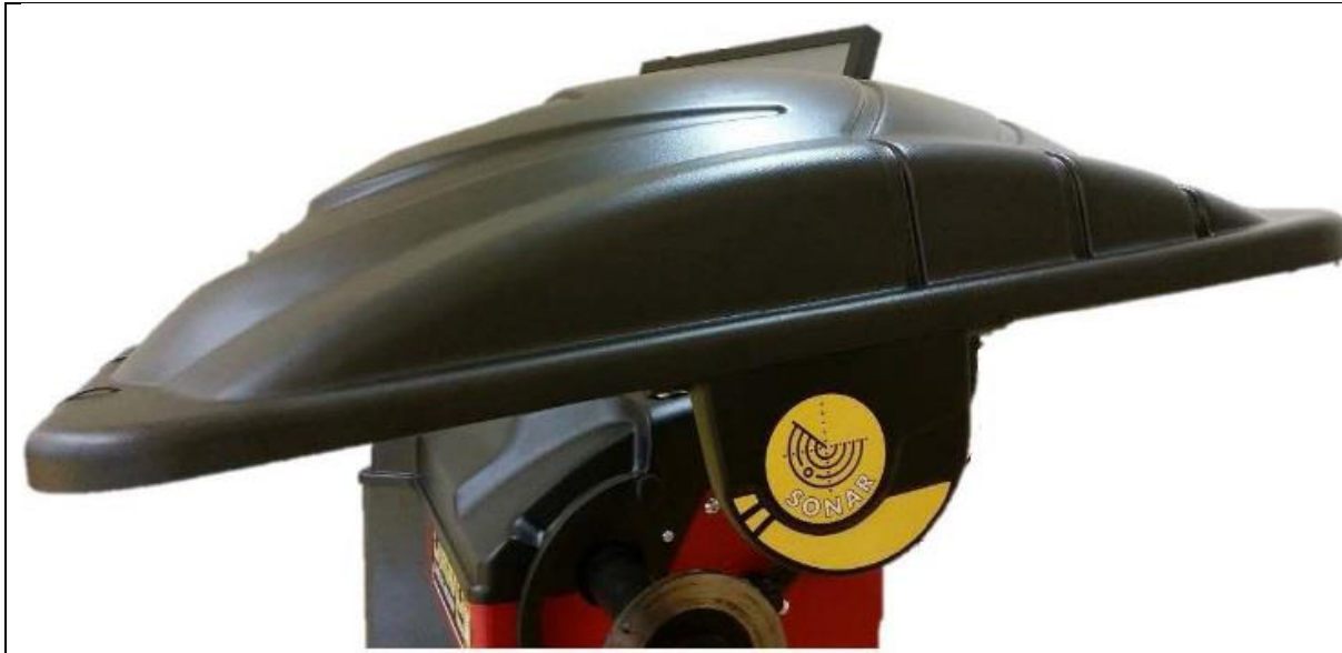
Figure F6.26: Once the device is mounted on the pipe, fit the plastic carter as described on the 6.3.
