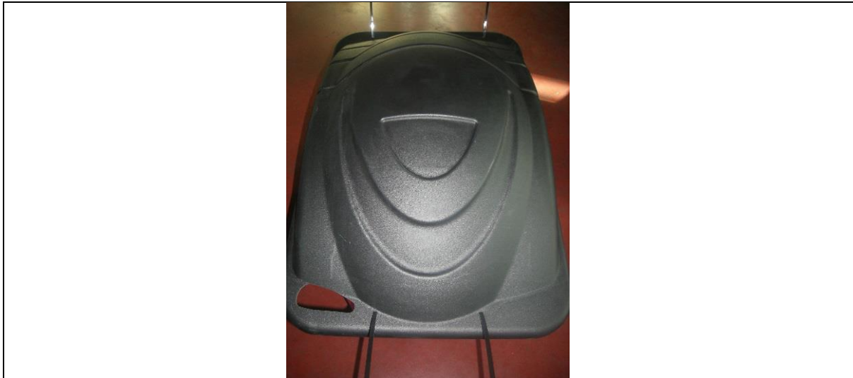
Figure F6.19: Secure the wheel guard to the tube using the relative ties.
