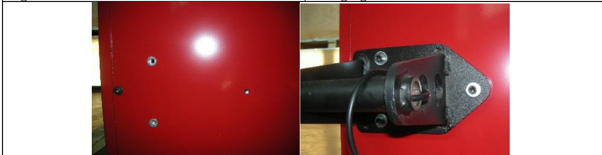
Figure F6.11 and Figure F6.12: There are holes at the back of the wheel balancer to attach the external sensor. Place the flange of external sensor on the three holes.
