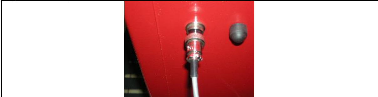
Figure F6.14: Connect the cable of the external sensor to the machine and screw on the connector.
