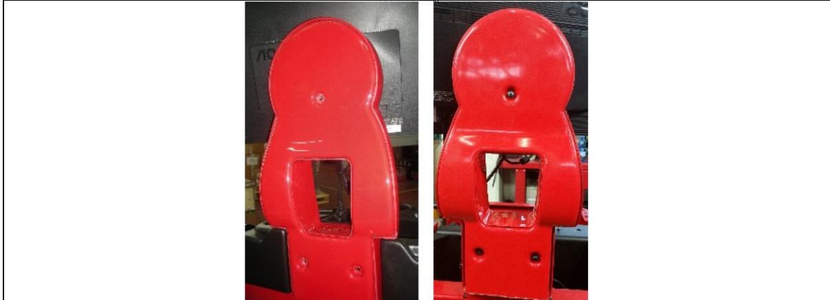
Figure F6.8 and Figure F6.9: Fix the rear plastic cover onto support with no. 3 M6 screws.
