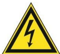
This sign is a reminder that the power supply to the housing must be switched off and locked so that it is secured against accidental switching on.
