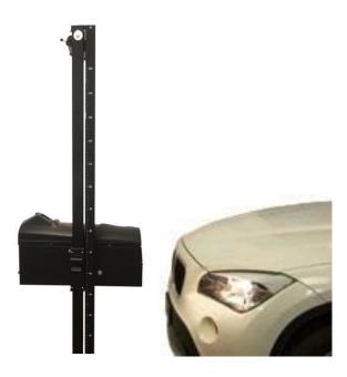
Switch the laser on by pressing the button on the side of the optical box. The laser beam will be projected from a point corresponding to the center of the lens, and will help you to align it with the center of the headlight
