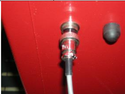
Picture F6.19: Square the external sensor using a level. Tighten the 3 M6 screws.
