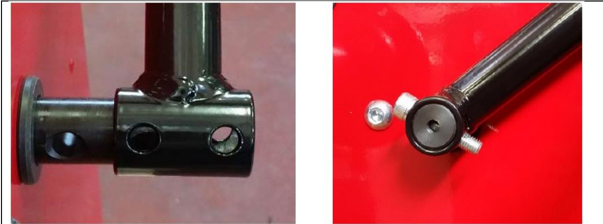
Picture F6.3 and Picture F6.4: Place the tube inside the relative pin and secure it with 2 M8 bolts.
