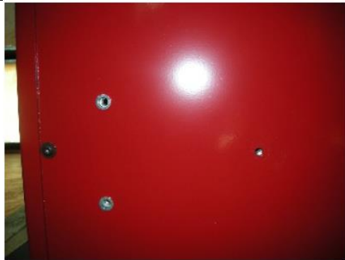
Picture F6.17 and Picture F6.18: There are holes at the back of the wheel balancer to attach the external sensor. Place the flange of external sensor on the three holes.
