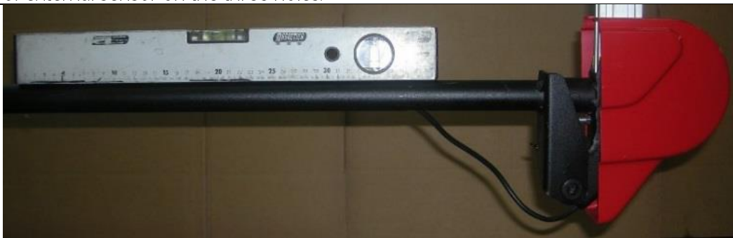
Picture F6.19: Square the external sensor using a level. Tighten the 3 M6 screws.
